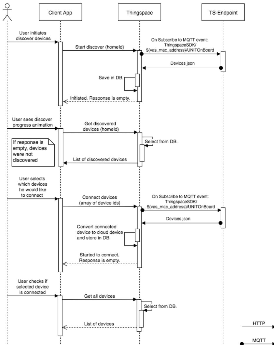
Any device interaction must first be enrolled by the host device into ThingSpace. The parameters for updating device property include device ID, capability ID and property value via HTTP request to ThingSpace Cloud. The Cloud will trigger MQTT command to TS-Endpoint UNIT for property update. After change property action was submitted ThingSpace Cloud returns response to Client Application with property update status.
